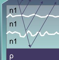
Multiple rough bragg layers With differents parameters
