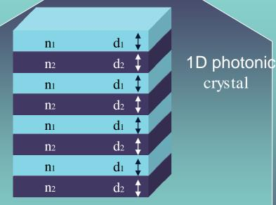
periodic arrangement of thin layers with distinct optical indices and widths
