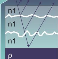
Multiple rough bragg layers With differents parameters
